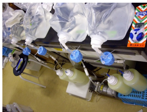
Fig. 2.4 Filtration of river water for water chemistry and DNA analysis.
